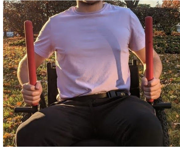
b) Grabbing the bottom of the levers is like high gear and is good for smooth ground. Push through long strokes to move quickly.
