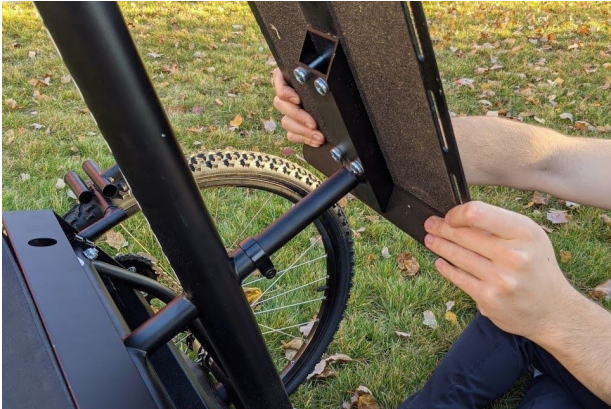
c) Slide the footrest tube into the frame until it is at an appropriate height.
