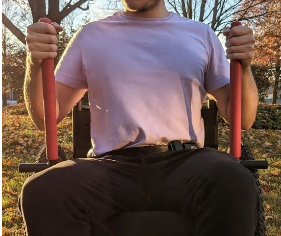
a) Grabbing the top of the levers is like low gear and is good for hills and tough terrains Use many small, alternating lever strokes to climb hills.
