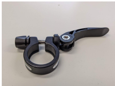
d) Orient the clamp so that the lip is at the bottom.
