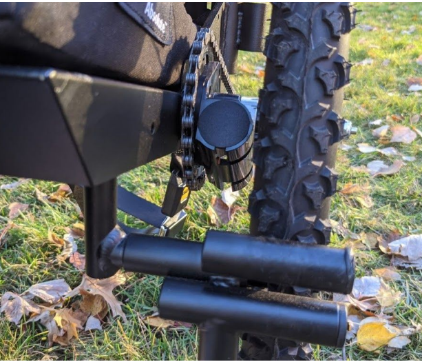
a) If the endcap is visible, rotate the coupling.
