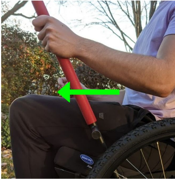
a) Push the lever away from the wheel.
