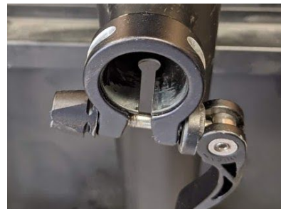
e) Slide the clamp onto the frame.
