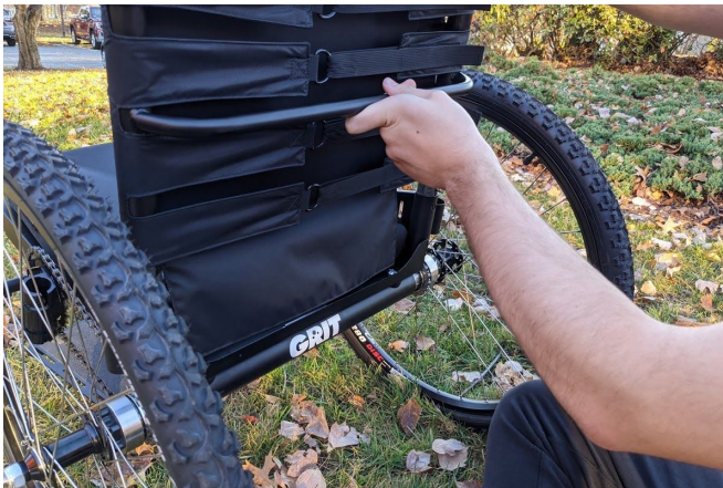
b) Hold both buttons in while pulling upward on both sides of the seatback.
