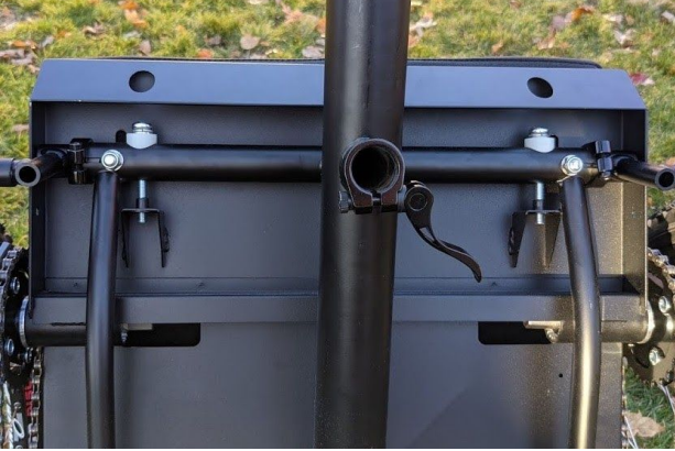
a) Ensure the footrest clamp is open and loose enough for the footrest to slide in easily.
