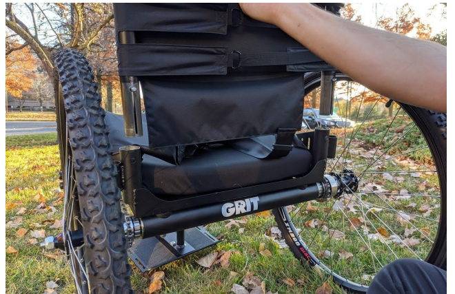
c) Continue pulling upward on both sides of the seatback until it is released.
