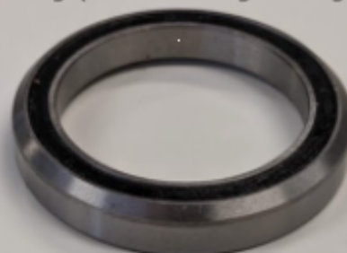
#8: Bearing (note the angled edge)
