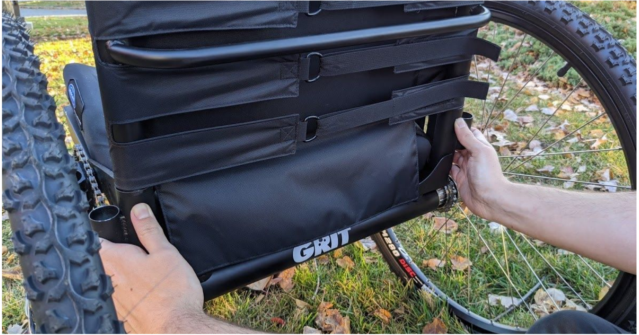
a) Simultaneously push in the buttons on both sides of the seatback.
