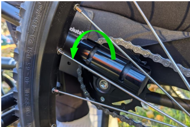
c) Rotate the lever in the coupling (as shown above).
