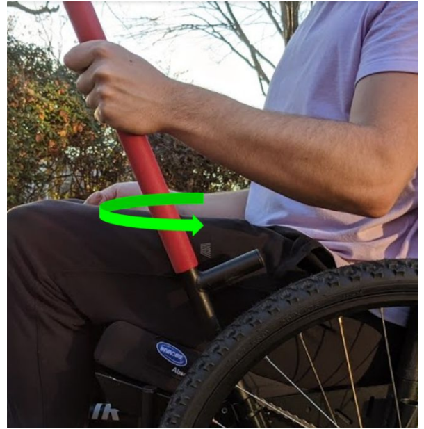
b) Rotate the brake bar toward yourself.
