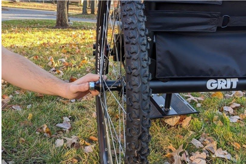
a) Grab the wheel near the hub and push the axle button inward.
