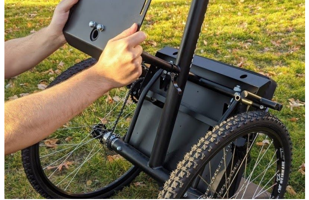
b) Insert the footrest tube with the footrest facing forward.
