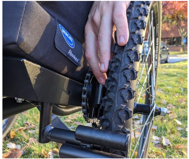
b) If the lever hole is inaccessible, rotate the coupling.
